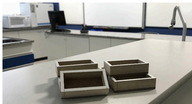
Figure 3: Brick molds made from plywood in the Colégio Dante Alighieri's laboratory.
