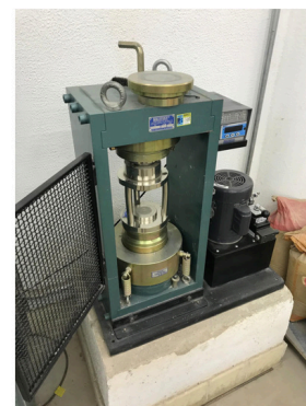
Figure 11: Hydraulic press used for brick compression tests (brand: Solotest).
