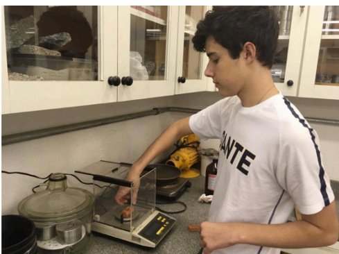
Figure 12: Determination of the mass of bricks in PUC-SP laboratory analytical balance.
