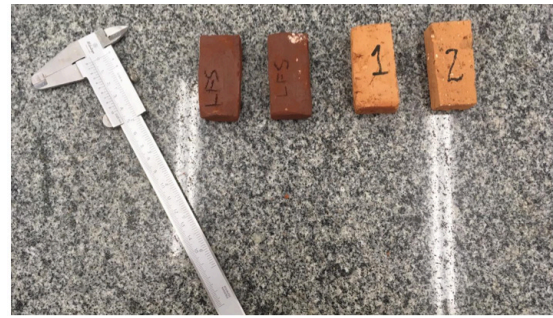
Figure 8: Waste bricks and common bricks after cutting in the civil engineering laboratory at PUC-SP.
