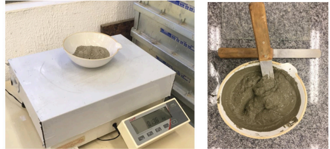
Figure 9: Cement being weighed on the scale and the cement mass prepared after adding water.
