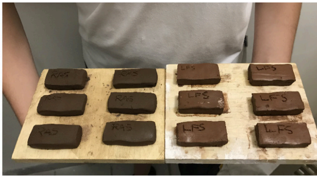
Figure 4: Mini bricks made from Samarco waste. On the left: sandy residue (RAS), and on the right: flotation mud (LFS).
